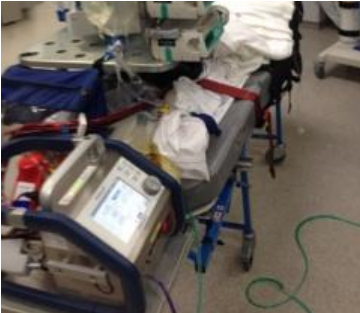
Figure 5 - ECMO attachment plate and device attached in its bracket onto the plate in Fixed Wing
